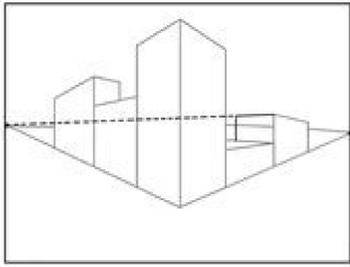
19. Connect the corner to the left vanishing point with an orthogonal line. Show the edge of the building with a transversal line.
